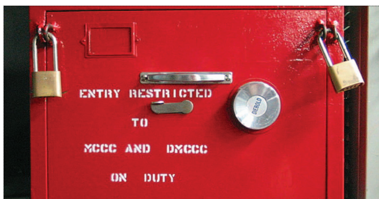
Figure 3. Principle of separation of privilege. Launch codes for Titan II nuclear missiles were stored in this safe. The two-person launch team had to work together to unlock the codes and launch the missile; neither could launch the missile independently. (Photo by the author, courtesy of the Titan Missile Museum.)
